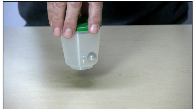
Swirl the control cup slowly to make the control magnet orbit inside the cup. Swirl either clockwise or counter-clockwise, whichever direction feels more natural to you.
